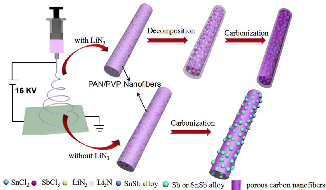
Fig. 1. Schematic illustration of the fabrication process of SnSb@N-PCNFs composites.
